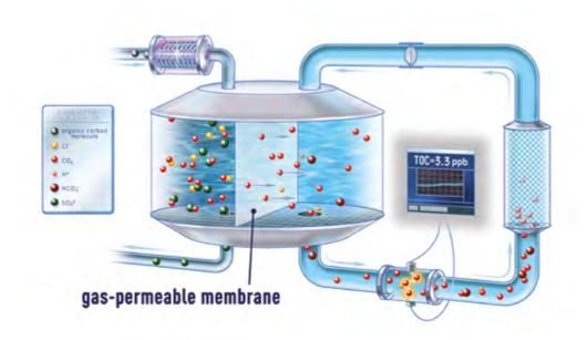
Gas-permeable membrane selectively passes only the CO<sub>2</sub> produced from oxidized organics, preventing acids, bases, and halogenated compounds from interfering with the measurement.
